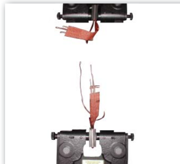
Tearing strength of fabrics according to ASTM D 2261
