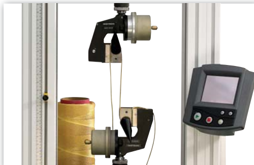
Tension test of single stranded yarn according to ASTM D 2256
